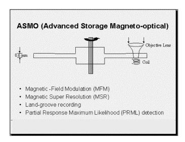
As shown in the figure above, a single sided disk has a small magnetic coil close to the recording layer. By using a small coil it is possible to switch the magnetic field at the data rate and achieve direct overwrite.
